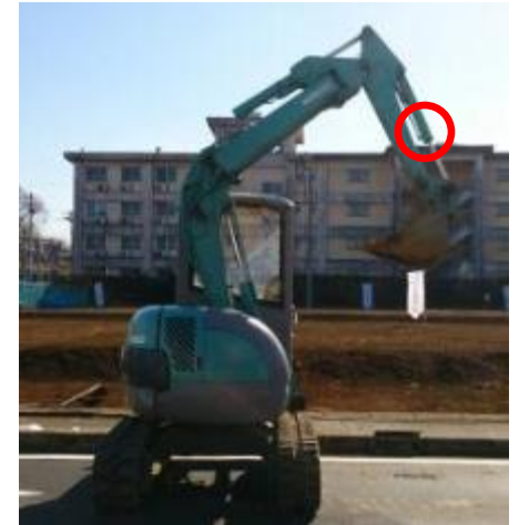
Slide ring of the cylinder
